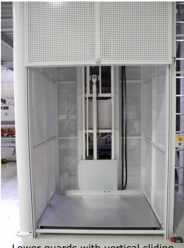
Lower guards with vertical sliding gate and safety electric lock
